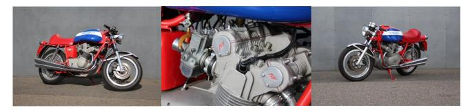
Launched in 1970, the MV Agusta 750 S was hand-built, expensive and, with only 583 units built, correspondingly rare. The MV 750 S was developed from the MV Agusta 4C 600cc. The engine was bored out to 743 cc and boosted to 72 hp with four Dell'Orto carburetors. The color scheme of the 750 S was unique and kept in red, white and blue. Today, it is a highly sought-after machine for MV collectors.
